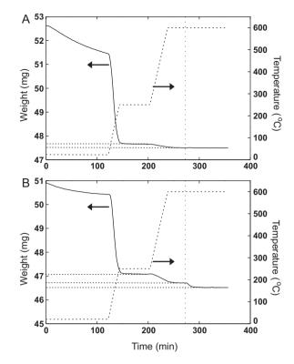
**Fig. 4.** Thermogravimetric profiles for (A) PtH-MFI and (B)  $Pt/Al_2O_3$  catalysts after 25 and 24 h of the reaction, respectively. Reaction conditions are given in the legend of Fig. 2. TGA procedure is described in Section 2.2, and the vertical dotted line corresponds to the switch from the nitrogen to the air flow.
