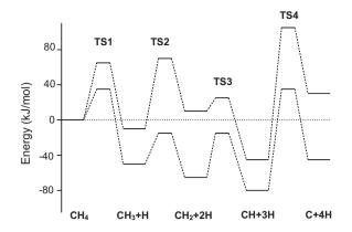
**Fig. 1.** Reaction energy diagrams for transformation of methane into carbon and hydrogen chemisorbed on flat Pt(111) terraces and stepped Pt(110)( $1 \times 2$ ) surfaces. All energies are referenced to methane in the gas phase and the clean surfaces. The top diagram for the flat Pt surface is based on the data in Ref. [33], and the bottom diagram for the stepped Pt surface is based on the data in Ref. [34]. TS stand for transition state.
