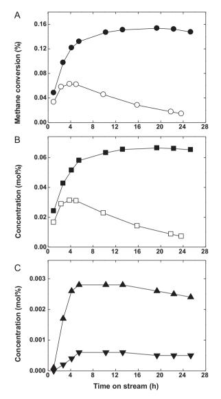
**Fig. 2.** Effect of time on stream on methane conversion and product formation over PtH-MFI (solid symbols) and Pt/Al<sub>2</sub>O<sub>3</sub> (open symbols) catalysts: (A) Methane conversion  $(\bullet, \bigcirc)$ , (B) concentration of ethane  $(\blacksquare, \Box)$ , and (C) concentrations of benzene ( $\blacktriangle$ ) and toluene ( $\blacktriangledown$ ). Reaction was carried out at 370 °C with pure methane as a feed and at weight hour space velocity of 1.26 h<sup>-1</sup>.
